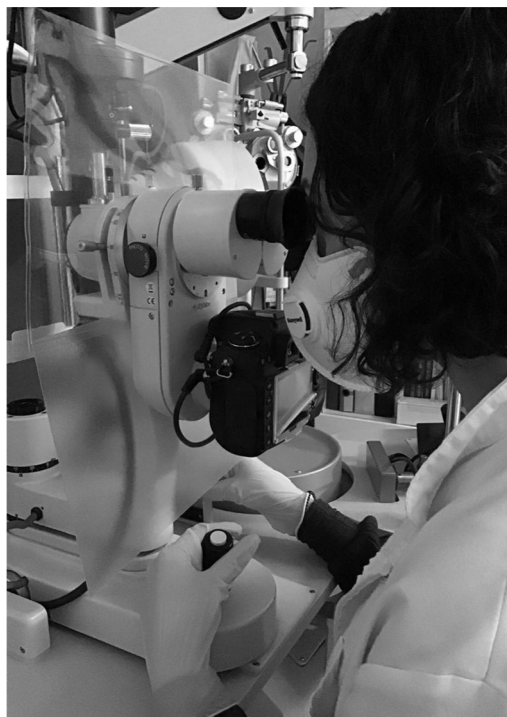
Fig. 2. A large clear plastic sheet, working as a protective shield, has been cut and placed between the ocular and slit lamp [9,10].
